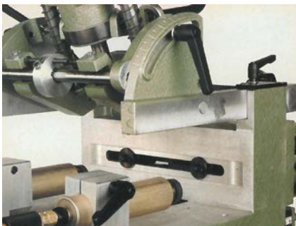
Swiveling scale for upper unit, pneumatic tensioning device, resilient miter stop
